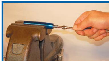
STEP 2 Flare braid using a twisting motion.
